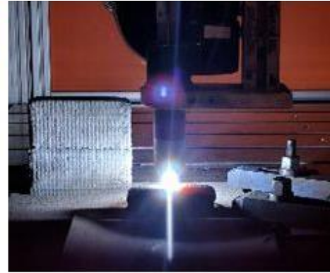
Figure 10: Main results obtained with Powder Metal Deposition process
