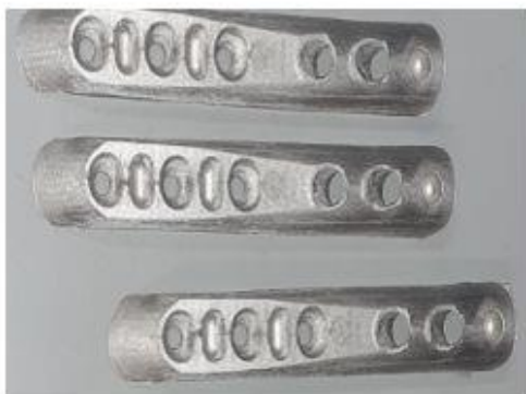
New MIM production route developed for a medical prosthesis (IDONIAL)
