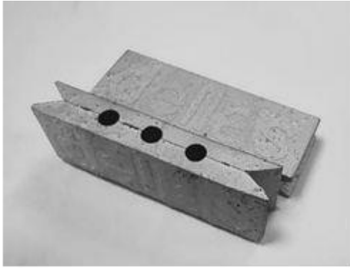
New alloy and new MIM feedstock developed for cutting tools segments (MBN, Tecnalía & DELLAS)
